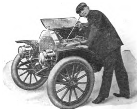
Fig. 2—How the Sonoscope operates
